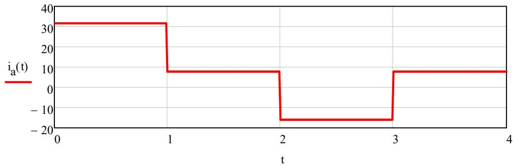
$$e(t) := \omega(t) \cdot \Psi_{fn} \quad u_a(t) := \omega(t) \cdot \Psi_{fn} + R_a \cdot i_a(t)$$
