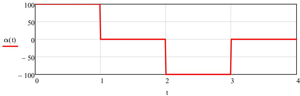
$$m_e(t) := m_m(t) + \Sigma J \cdot \alpha(t) \quad i_a(t) := \frac{m_e(t)}{\Psi_{fn}}$$
